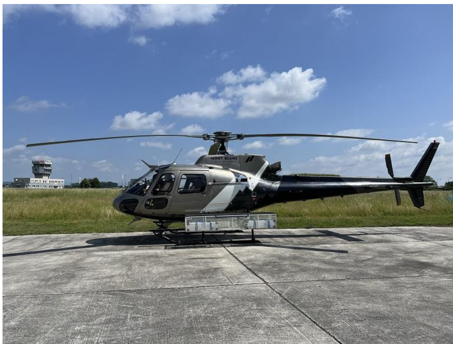
Fig. 14 AS350 for the AGC24, equipped with lateral basket containing 2 x 4 liters NaI units
