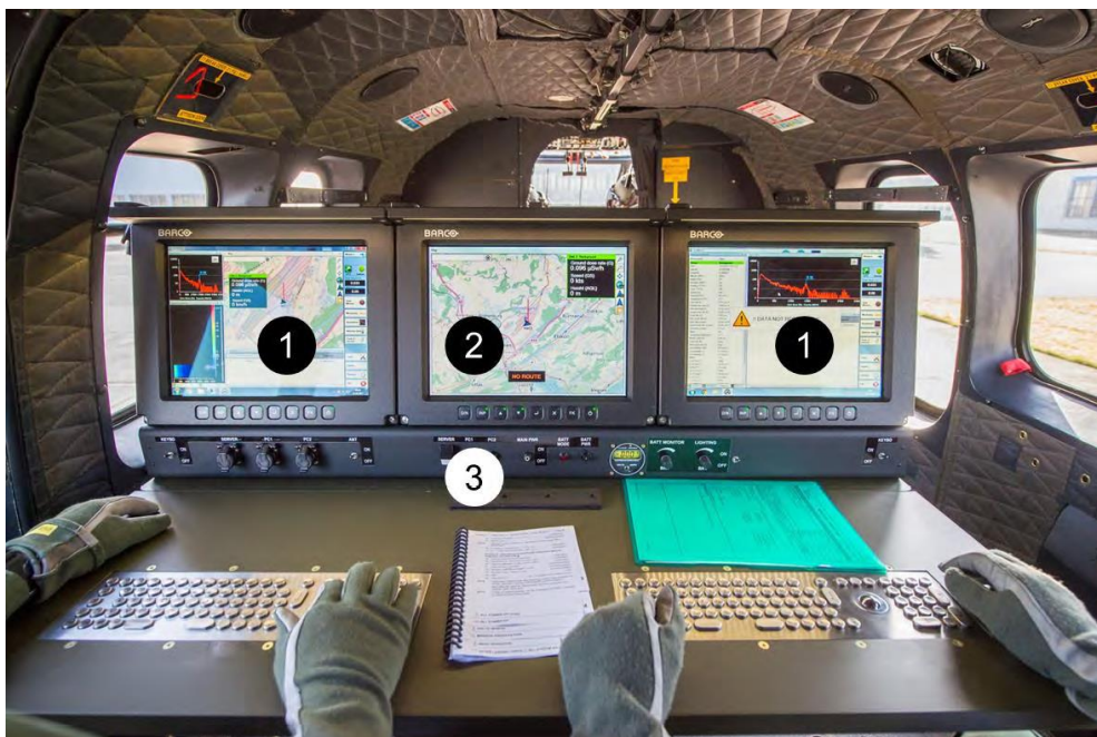
Fig. 9 Operator console of the RLL system. 1. Displays of the client computers. 2. Common display (mirrored in the cockpit). 3. Control panel with switches for power, lighting and communication and USB ports for file exchange.
