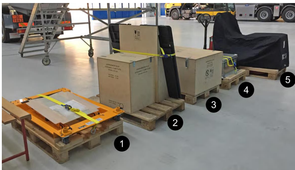
Fig. 8 Components of the RLL system. 1. Lifting platform for the installation of the detection container. 2. Floor plates and accessories case. 3. Monitors and operator console. 4. Detection container. 5. Operator seats and equipment rack.
