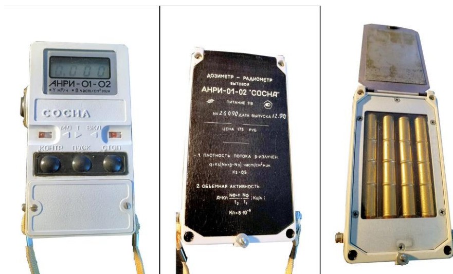
Figure 10. Anri 01-02 "Sosna" detector (photo by Karel Svoboda, CC BY-SA, Flickr.com)
