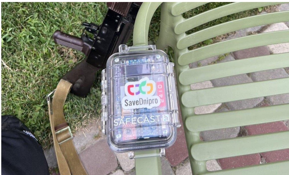
Figure 32. A #bgeigies4ukraine bGeigie Nano in the field (photo by Pavlo Tkachenko, SaveDnipro)
