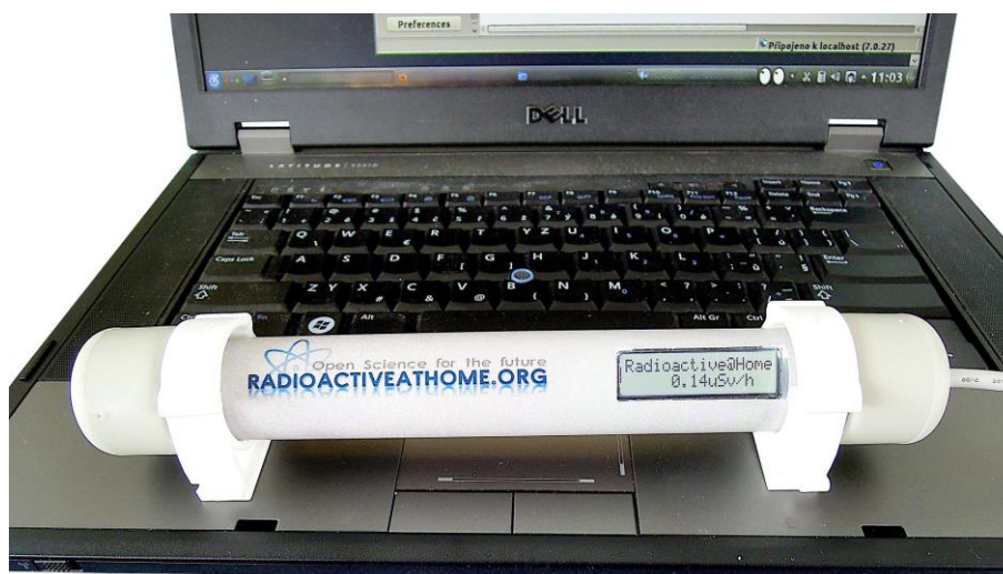
Figure 22. Radioactive@Home detector (photo by Jan Helebrant, CC BY-SA, Flickr.com)
