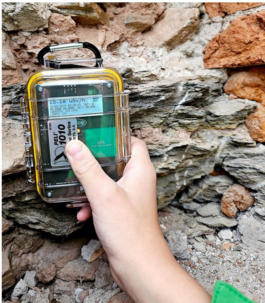
Figure 28. CzechRad detector during the field measurements (photo by Marie Davidková, CC BY-SA, Flickr.com)
