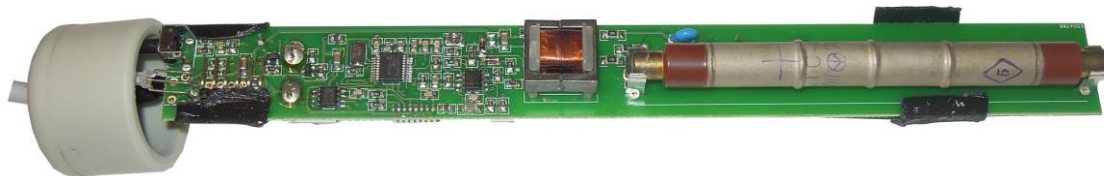
Figure 23. Inner part of the detector (photo by Jan Helebrant, CC BY-SA, Flickr.com)
